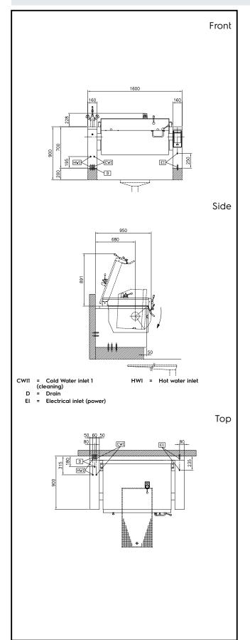
Electric Supply voltage: 400 V/3N ph/50/60 Hz Total Watts: 20.6 kW Installation: FS on concrete base;FS on feet;On base;Standing Type of installation: against wall **Key Information:** Working Temperature MIN: 50 °C Working Temperature MAX: 250 °C Vessel (rectangle) width: 1050 mm Vessel (rectangle) height: 326 mm Vessel (rectangle) depth: 558 mm External dimensions, Width: 1600 mm External dimensions, Depth: 900 mm
